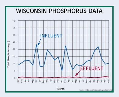
We use a chemical dosing system, low horsepower pumps and mixers that make operation easy. Phosphorus is precipitated chemically by the addition of coagulants, including alum or ferric chloride. Precipitation causes contaminants that are either dissolved or suspended to settle out of solution as solid floc particles that are removed along with waste biological sludge. Our system is low cost and reliable.
